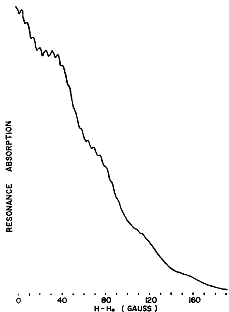
FIG. 6. Absorption spectrum (integrated recorder trace) of F centers in neutron-irradiated \text{Li}^6\text{F} with \text{H} along [111] . Only the high-field half of the resonance is shown.
